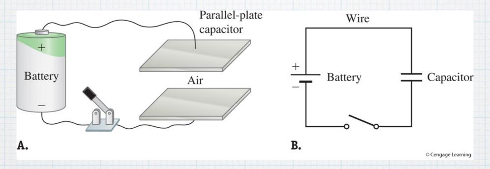
When the switch is closed the capacitor charges until there is an accumulation of +Q charge on the top plate and -Q on the bottom. The potential difference across the capacitor reaches the same value as the voltage of the battery
