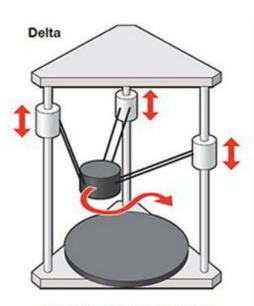
Printer head can move in any direction quickly.
