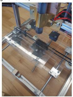
Step 10: Assemble the large rail as shown in the photo.
