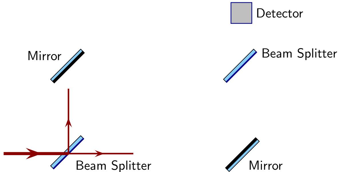
First beam splitter transmits 50% of incident light, reflects 50% of incident light.
