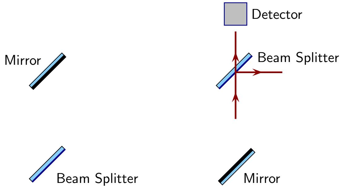
Second beam splitter transmits 50% of incident light, reflects 50% of incident light.
