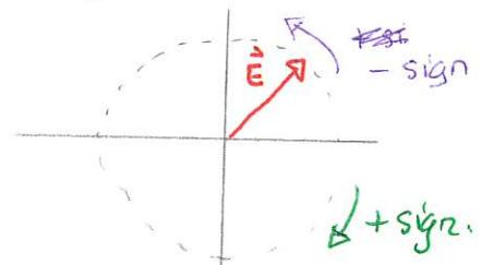
3) elliptical polarization If  $\delta_y = \delta_x \pm \pi/2$  and  $E_{ox} \neq E_{oy}$  then
