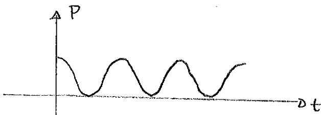
We can determine and observe the average rate at which power flows. For a sinusoidally oscillating function we can average over one period,  $T$ .
