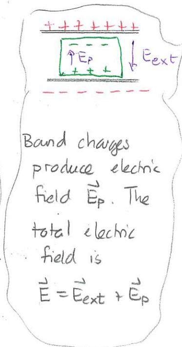
We aim for methods to compute the total electric field produced by the free and bound charges. This will be facilitated by an auxiliary quantity called the electric displacement
