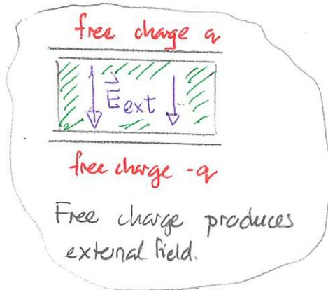
External field induces polarization in material
