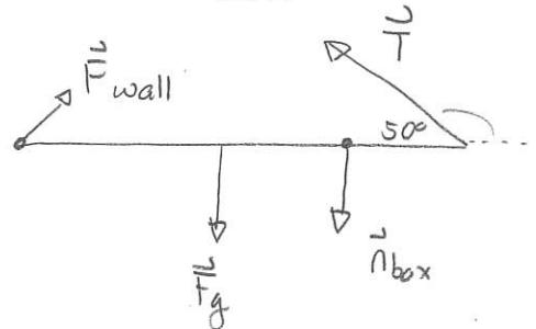
$$\text{Rope: } \phi = 180^\circ - 50^\circ = 130^\circ \quad \tau_{\text{rope}} = rF \sin 130^\circ$$
