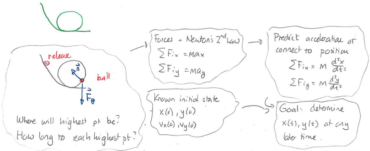
Challenge here:  $\rightarrow$  normal force depends on position - need to know position (at time  $t$ ) to determine normal force and find acceleration at time  $t$ .  $\Rightarrow$  acceleration depends on location
