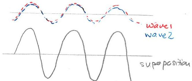
2 Destructive interference - here a crest aligns with a trough
