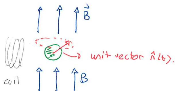
is a unit vector rotating about  $\vec{B}$  with angular frequency  $\frac{qqB}{2m}$ .
