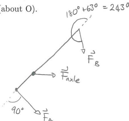
Force axle:  $\tau_{\text{axle}} = \underbrace{F_{\text{axle}}}_{=0} r_{\text{axle}} F_{\text{axle}} \sin \phi = 0\text{N.m}$
