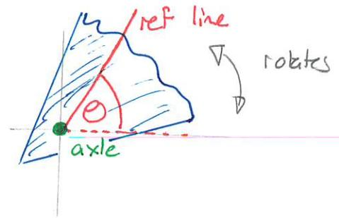
Angular position  $\leadsto \theta$  measured in radians counterclockwise from a reference line.
