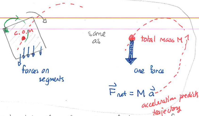
Provided that the object does not rotate then the motion of the center of mass is sufficient to describe the object's motion since at each instant every point has the same velocity.
