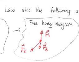
Relates to acceleration = Fretx = Fix+Fix+ ... = Max Frety = Fig + Fzy + ... = may
