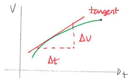
Acceleration = slope of  $v$  vs  $t$  graph
