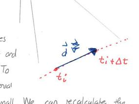
from to tito that whose At is very small. We can recalculate the average velocity over this interval. Take Dt -DO gives a velocity at ti
