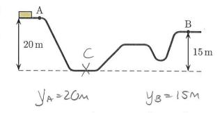
11 +1 +1 +1 = 1 500kg ×9.8 m/s² × 15 m = 1 500kg × (20m/s) 2 + 500kg ×9.8 m/s² × 20m
