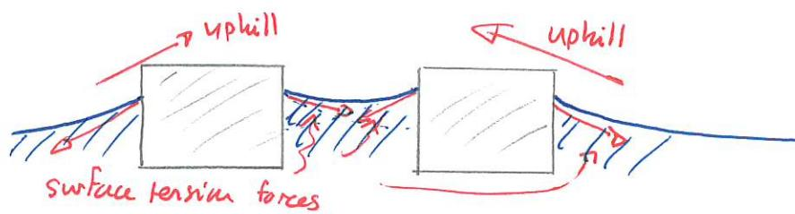
The distortion is illustrated and the objects tend to float uphill. They will therefore appear to attract each other. A detailed analysis considers surface tension forces and buoyancy
