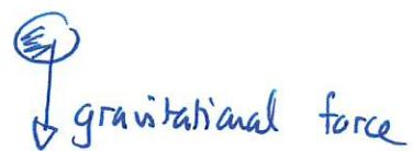
$$\text{acceleration} = \frac{\text{net force}}{\text{mass}} = \frac{\text{gravitational force}}{\text{mass}}$$
