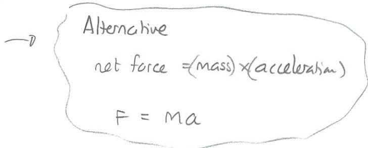
Note that the net force does not determine velocity. It determines how velocity changes
