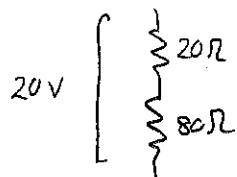
$$\Delta V = I R_{eq} \quad R_{eq} = 20\Omega + 80\Omega \\ = 100\Omega$$
