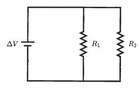
The power dissipated by each resistor is smaller than that for the battery; the power dissipated by resistor 1 is larger than that dissipated by resistor 2.
