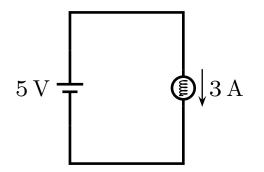
The current through the bulb and potential difference across the battery are indicated. The wires offer negligible resistance.
