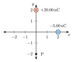
b) Determine the magnitude of the net electric field at the point labeled P.
