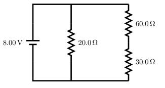
b) Suppose that  $20.0 \Omega$  resistor is replaced by a  $10.0 \Omega$  resistor. Explain whether the current through the  $60.0 \Omega$  resistor increases, decreases or stays the same as a result of this change.
