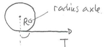
$$I = I_{\text{disk}} + I_{\text{axle}} = \frac{1}{2} M_{\text{disk}} r_{\text{disk}}^2 + M_{\text{axle}} r_{\text{axle}}^2$$
