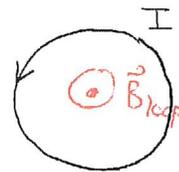
The electron will produce a magnetic field opposite to that of the external field. This diamagnetic effect is commonplace and important in applications such as NMR.
