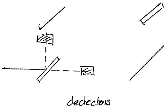
With the right type of light and a sufficiently low intensity we will observe that only one of these detectors registers. Then repeated runs of this show that we cannot predict which one. In this way it appears that light:
