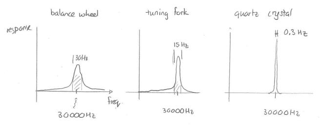
Generally for a quartz crystal the range of frequencies in which it operates is 100000 to 1000000 of its true natural frequency. This is considerably less than for most mechanical oscillators. Therefore it will be inherently superior in maintaining a precise frequency.
