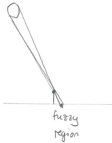
Here the fuzzy region will be smaller for a lower gnomon. However, the distance moved by the shadow will be smaller during a fixed interval and harder to measure accurately.
