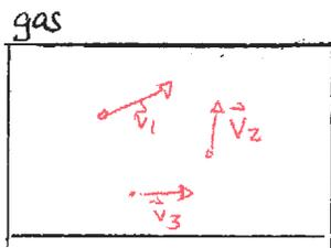
molecules with velocities. For molecule  $i$  energy  $K_i = \frac{1}{2} m v_i^2$
