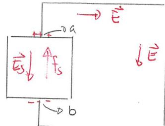
$$\Rightarrow - \int_{\text{source}} \vec{f}_s \cdot d\vec{l} = - \int_{\text{wire } a-b} \vec{E} \cdot d\vec{l}$$
