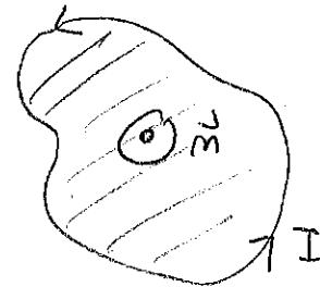
where the integral is over any surface that bounds the current loop. The direction of  $d\vec{a}'$  is determined via the r.h.rule and the current direction.
