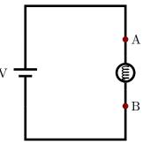
c) Suppose that the battery can provide 9.6 kJ of energy. Determine the amount of time for which the battery could operate in this circuit.
