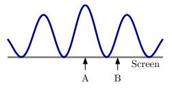
b) Suppose that in a short period of time 8000 photons arrive at A. Approximately how many will arrive at B during the same period of time?
