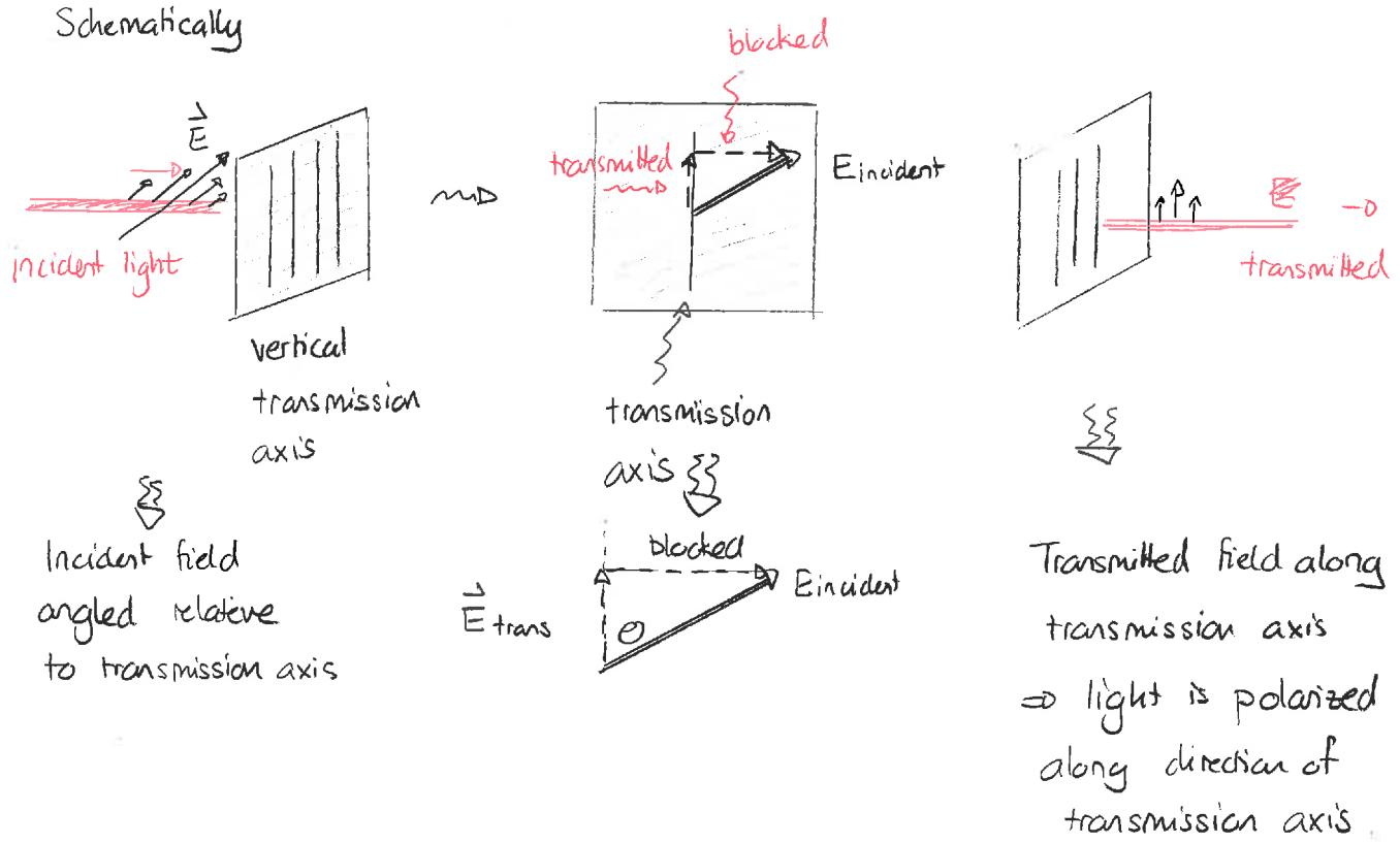
Transmitted field along transmission axis
