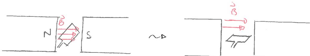
Because the angle between field + loop changes, the flux changes with time and this induces an EMF and hence a current
