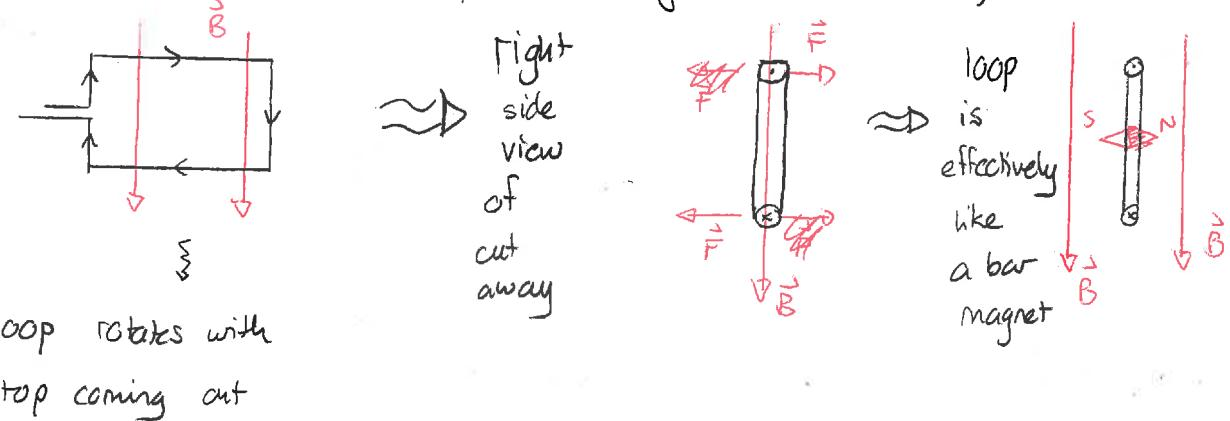
The fact that the loop is like a bar magnet and has a north and south pole leads to the nomenclature that it is a dipole. We see that the forces cause the dipole to align with the field
