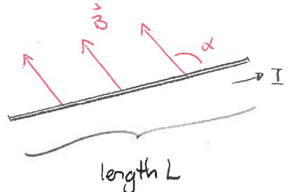
This rule is devised so that the direction of the force depends only on the current direction and does not require any accounting for the sign of the current carrying charge.
