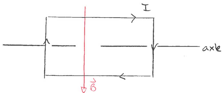
By analyzing the forces on all sides we see that the loop rotates about the indicate axle.
