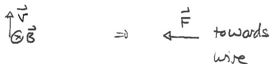
$$\begin{aligned} F &= |q|vB \sin\alpha &= 6.0 \times 10^{-9} \text{ C} \times 3.0 \times 10^6 \text{ m/s} \times 2.0 \times 10^{-3} \text{ T} \sin 90^\circ \\ &= 36 \times 10^{-6} \text{ N} \end{aligned}$$
