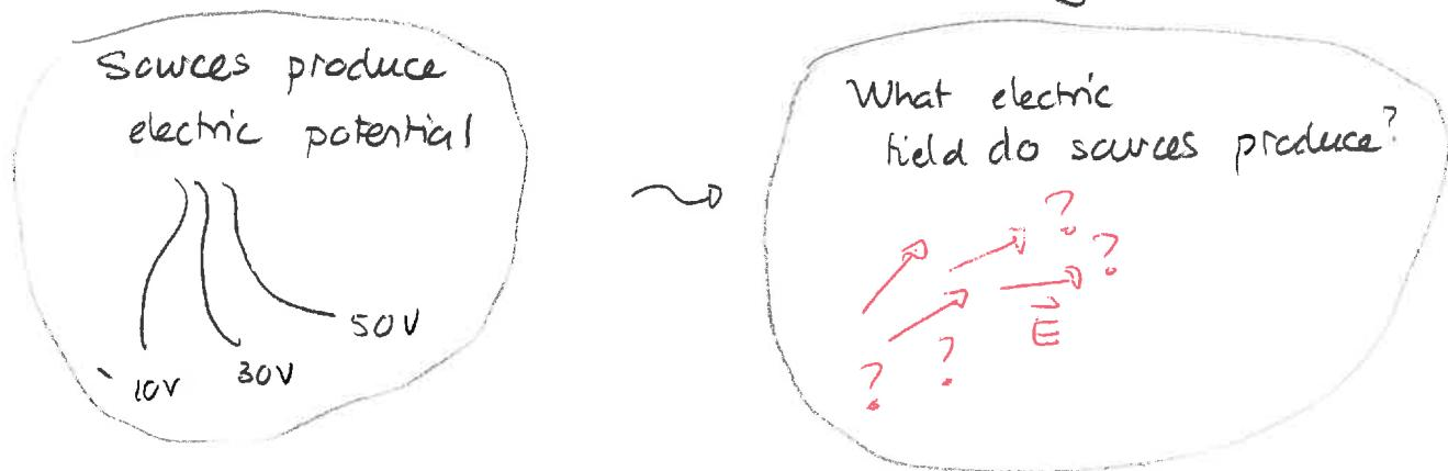
The exact relationship requires calculus. But we can elucidate some ideas by considering a positive probe charge in a potential. We know that when released, the particle will move in direction of decreasing potential. Its speed will increase. Thus acceleration will point as illustrated. This gives the electric force. But  $\vec{F} = q\vec{E}$  and  $q > 0$  gives the indicated electric field direction.
