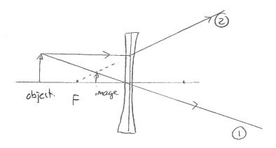
The intersection point will always be somewhere along the dashed line. This lies between F and lens So image is always between left focal pt and lens.
