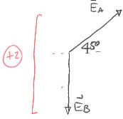
$$E_{A} = K \frac{|q_{A}|}{\Gamma_{A^{2}}} = 8.99 \times 10^{9} \text{Nm}^{2} \frac{|4.0 \times 10^{-9} \text{Cl}}{(0.07 \text{Im})^{2}}$$
