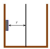
b) Determine an expression for the minimum angular velocity with which the drum must rotate so that the block does not slip.
