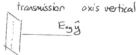
the system of light if it is perpendicularly polarized
