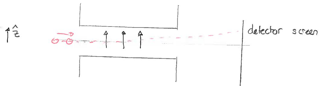
The deflection on the detector turns out to be proportional to the component of the spin along the magnetic field direction.
