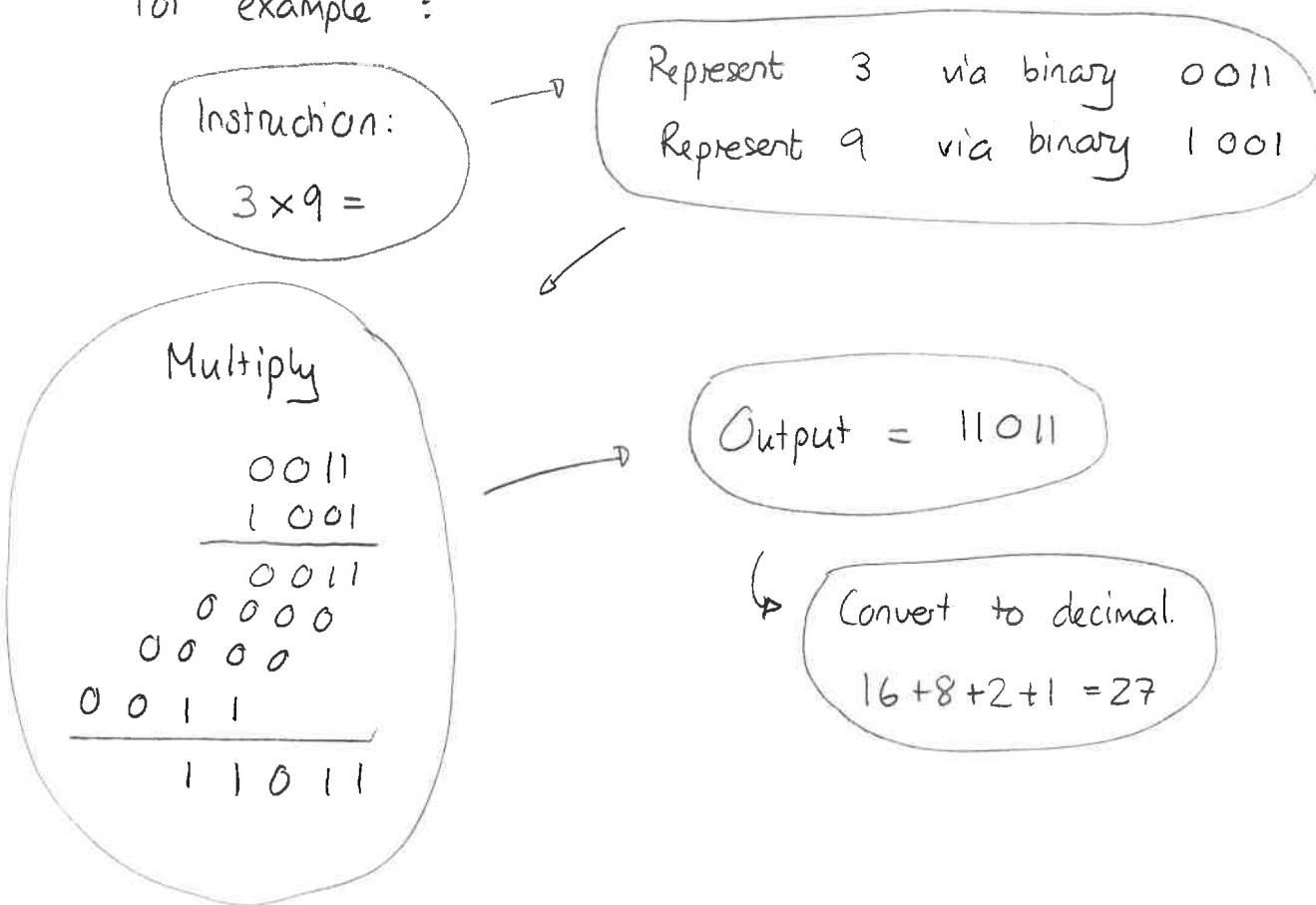
Hidden here are certain fundamental binary arithmetic operations on single bits. For example the operations
