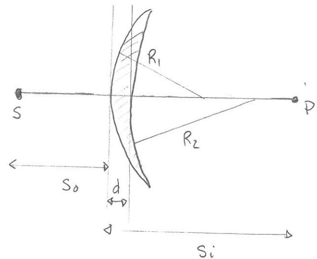
Proof: The first spherical surface (radius  $R_1$ ) produces an image at point  $P_1$ , where
