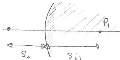
This would be true if the medium of the lens extended back. This serves as a virtual source for the second surface. We could reverse the analysis to say that there is another source  $S_2$  that would produce the rays that appear to pass through  $P_1$ . Then
