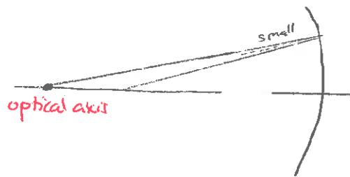
Consider, for the moment, a general case of a spherical surface of radius  $R$ . We consider a source  $S$  and ask: Where does the law of reflection predict that the ray will pass after reflection to the optical axis, which is a diametrical line through the center
