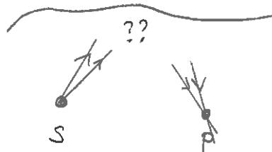
The only surface that produces a perfect image of a point source is an ellipse. The source must be at a focus of the ellipse for this to occur. The image will be produced at the other focus.
