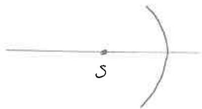
We will want to broaden this to find where approximate images are formed when the source is not at the center of the sphere. This will in general work when the spatial extent of the mirror is such that rays from the source make small angles of incidence at the reflecting surface.
