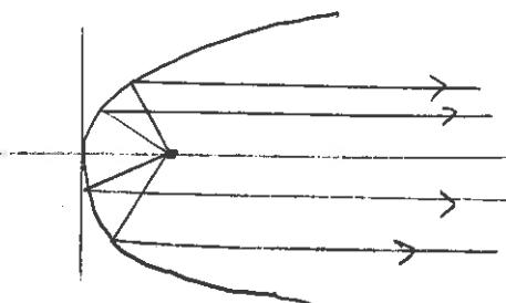
These parabolic mirrors form an image of an object that is infinitely far from the mirror. The object must be on the axis of the mirror and the image will be formed at the focus. An off axis object will result in an image formed elsewhere. And there will be some distortion in the image
