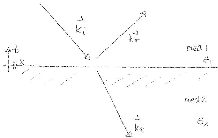
The plane of incidence is perpendicular to the surface that constitutes the interface. In the illustration the plane of incidence is the same as the plane of the page.
