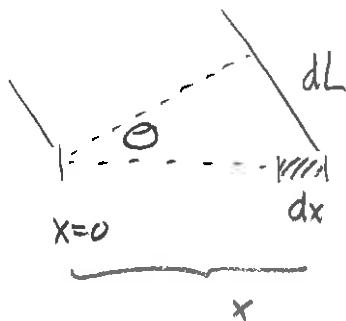
b)  $A \cos[kL + kx \sin\theta - wt] dx$  and  $z(t) = A e^{i(kL + kx \sin\theta - wt)}$
