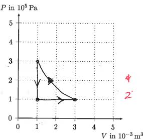
For isothermal PV = constant, Along this curve  $PV = 3 \times 10^2 \text{ J}$ So at end  $V = 1 \times 10^{-3} \text{m}^3 = 0$   $P = \frac{3 \times 10^2 \text{ J}}{1 \times 10^{-3} \text{ m}^3} = \frac{3 \times 10^5 \text{ Pa}}{1}$
