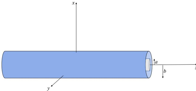
Notice that the surface charge is negative and of just the right magnitude so that the cable as a whole is electrically neutral.
